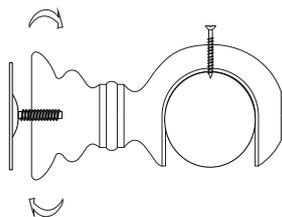
1. Remove the metal base plate from the bracket and fix to the wall in the correct position using the wall plugs and screws provided.
