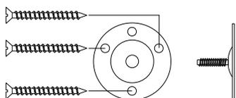
2. Screw the tieback stem onto the base plate until it is firmly against the wall.
