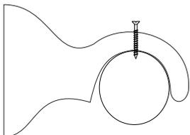
1. Mark the required position and secure to the wall using 2 x wall plugs and 2 x 50mm screws.
